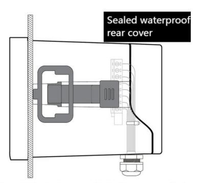
Insert the instrument into the square hole and fix it with the configured buckle.
