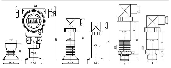
\*Unit is mm. Above is typical structures. Other structures and dimensions can be customized.
